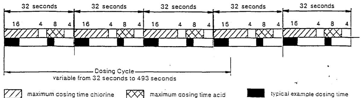
On the dosing cycle and dosing time knobs the scale of 1-16 is set to give the most appropriate cycle time and dosage to suit the individual pool. The diagram and table below shows the cycle timing and given values for various settings
